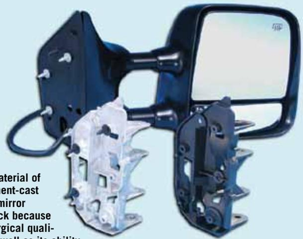
**Magnesium was the material of choice for this investment-cast telescopic trailer tow mirror mount for a pickup truck because of its superior metallurgical qualities and castability as well as its ability to provide a 3-lb. (1.36 kg) weight savings over aluminum.**
